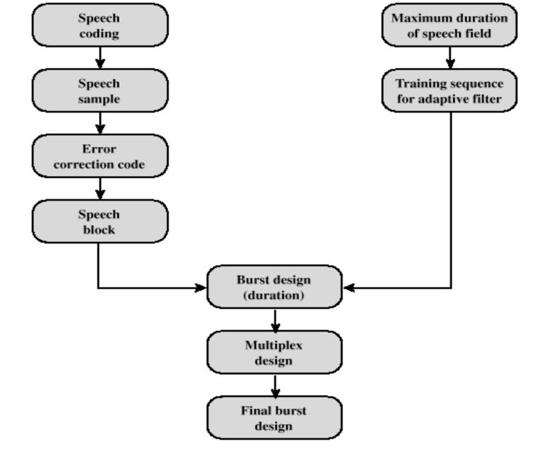
Figure 10.12 Steps in Design of TDMA Timeslot
