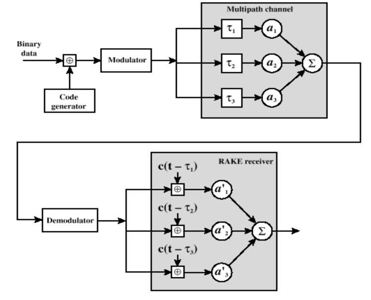
Figure 10.18 Principle of RAKE Receiver [PRAS98]
