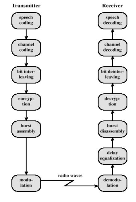
Figure 10.16 GSM Speech Signal Processing
